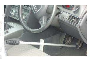
driver's seat and hold the brake pedal in a depressed position.
