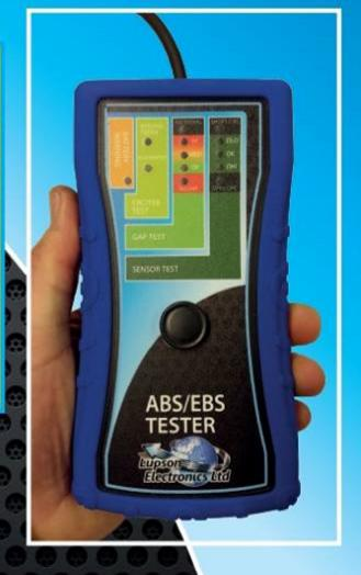
This tool is specifically designed to test the wheel speed ABS and EBS sensors. Simply plug into the sensor, press the 'ON' switch and wait for the 'SENSOR OK' LED to illuminate. Then spin the wheel. Results within 15 seconds.
