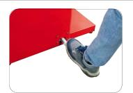
PEDAL LOCKING BRAKE (OPTIONAL) The pedal brake (G) facilitates wheel mounting on the machine and the counterweight application steps.
