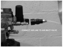
Connect quick release coupling on air line to male plug on air inlet on tank
