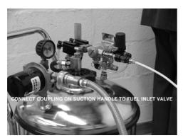
Connect female coupling on suction handle to fuel inlet valve (next to oil filter).
