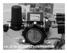
Make sure function switch is in oil depletion position.
