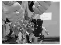
Attach handle assembly to fuel retriever using 4 screws supplied in the holding brackets welded to side of fuel extractor unit.
