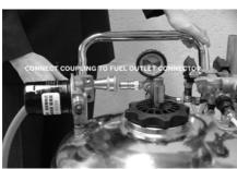
Connect quick release coupling on suction handle to fuel outlet.
