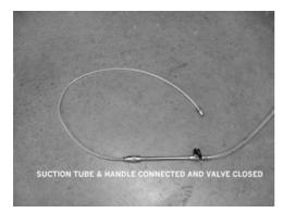
Make sure ball valve on suction handle is in closed position, i.e., 90 degree to tube.
