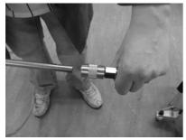
Attach to suction tube & handle using suction tube adapter
