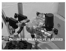
Before connecting tank to air compressor valve make sure air inlet valve is closed and also that pressure release valve is closed.
