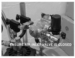
Before connecting tank to air compressor valve make sure air inlet valve is closed
