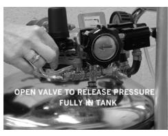
Release pressure in tank by opening up pressure release valve gently until pressure is released
