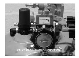
Ensure function switch is in oil suction position.
