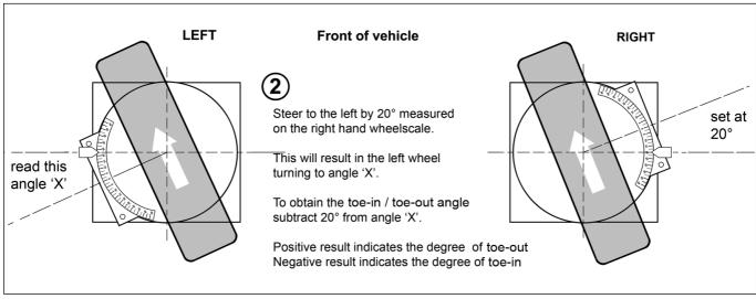
4.3 Measure the **WHEEL ANGLES** and the **TOE-IN/OUT ANGLES** for both left and right steering as described above and below. COMPARE YOUR READINGS WITH THE VEHICLE MANUFACTURER'S RECOMMENDATIONS.
