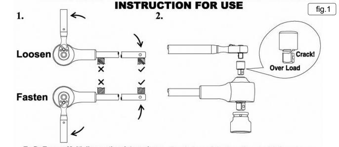
To fix Torque Multiplier as the picture above. Break-Away Adapter will protect it from harm.
