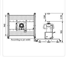
$<sup>\</sup>bullet\,$  The pit must be equipped with rails (100 x 100 x 10 mm)
