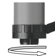
fig. 1 Screw lock ring fully onto pump.
