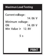
**Please Note:** Please do not turn off the engine during the test. Other electrical equipment should be turned off. If any electrical appliances in the car are switched on or off during the test, it can affect the accuracy of the test results.
